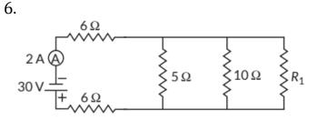
In the above circuit, if the current reading in the ammeter A is 2 A, what would be the value of  $R_1$ ? (Term II, 2021-22)
