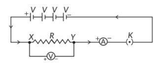
12. Ohm's law: It states that the potential difference V, across the ends of a given metallic wire in an electric circuit is directly proportional to the current flowing through it, provided its temperature remains the same. Mathematically,
