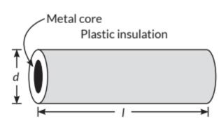
Plastic insulation surrounds a wire having diameter d and length I as shown above. A decrease in the resistance of the wire would be produced by an increase in the
