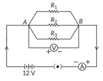
Here,  $R_1 = 10 \Omega$ ,  $R2 = 20 \Omega$  $R3 = 30 \Omega$  and V = 12 V
