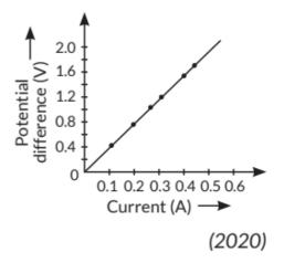
9. Study the V-I graph for a resistor as shown in the figure and prepare a table showing the values of (in amperes) corresponding to four different values V (in volts). Find the value of current for V = 10 volts. How can we determine the resistance of the resistor from this graph? (Board Term I, 2016)
