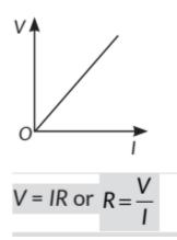
So, the slope of V-I graph at any point represents the resistance of the given conductor. As graph is a straight line, so it is clear from the graph that
